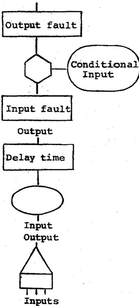
INHIBIT Gate: Input produces output directly when conditional input is satisfied.
