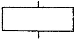
**Rectangle:** A fault event usually resulting from the combination of more basic faults acting through logic gates.
