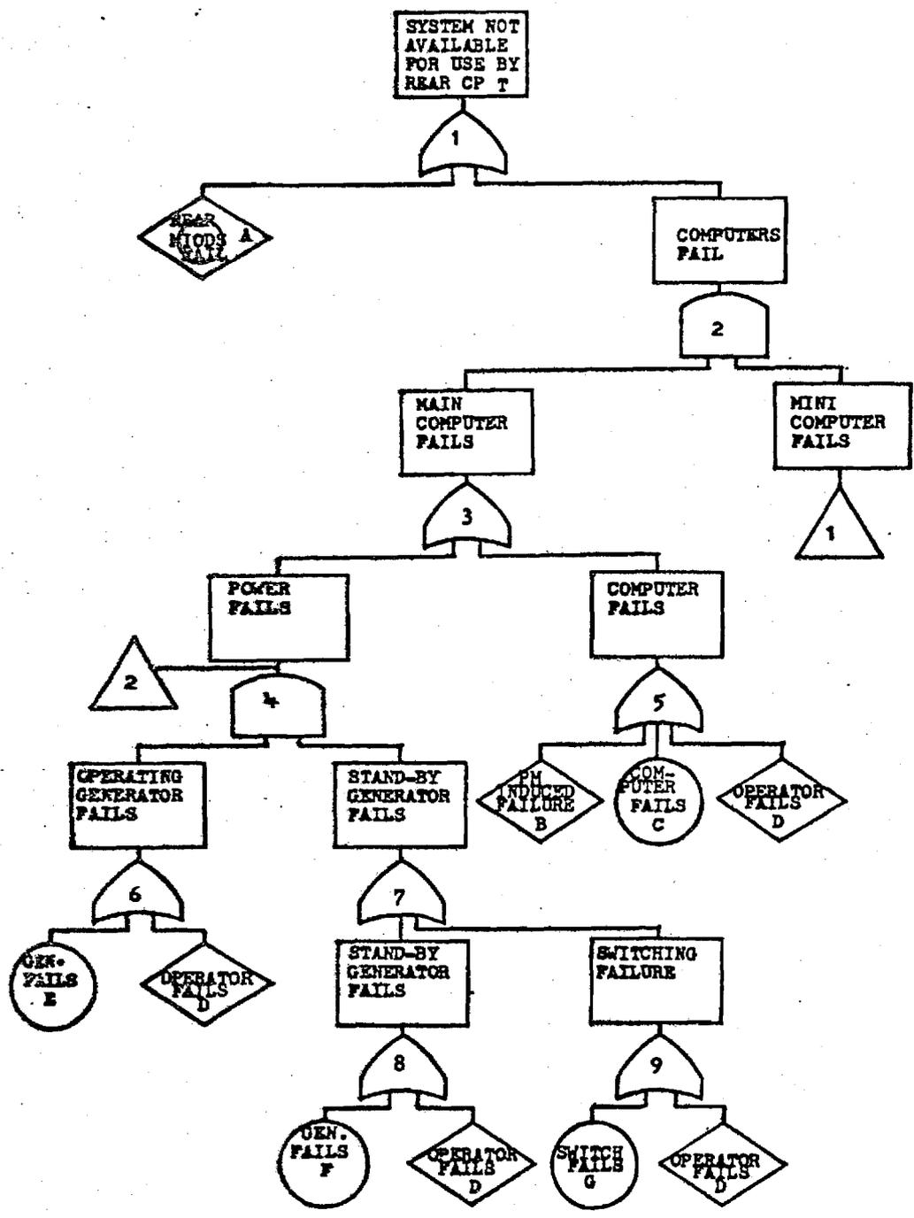
Figure 5. Fault Tree for C & C System
