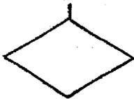
**Diamond:** A fault event not developed to its cause.
