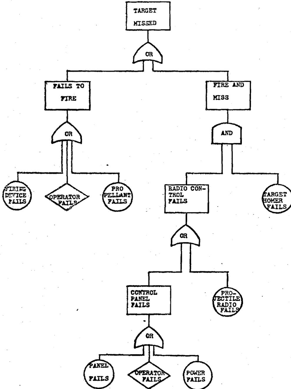
Figure 1. SIMGUN Fault Tree
