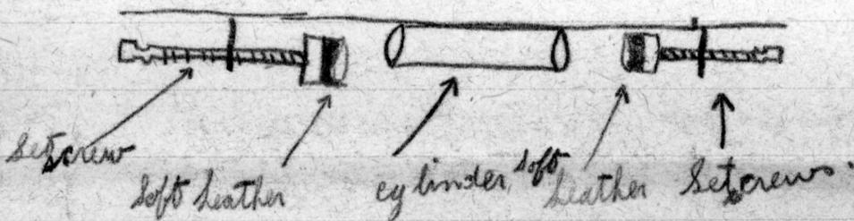
Cylinder works back and forth and setscrews are stationary leathers on end of set screws fall into openings on each end of cylinder as it works and takes away jar and lost motion, I heard Garrison speak to Fisher and Mr Coon about this, and I know if the leathers on machines are not properly cared for, the machines will be worn out just from the slam, banging it
