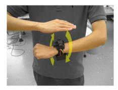
Figure 8. Around: move hand from body, over top and then around the wrist.
