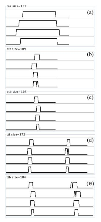
Figure 11. Representation of the signals for five gestures. (a) Cover all sensors. (b) One time forward. (c) One time backward. (d) Two times forward. (e) Two times backward.
