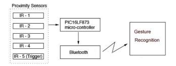
Figure 12. The Gesture Watch is composed of a PIC microcontroller which reads data from 5 IR proximity sensors. The PIC sends the sensor data wirelessly using a Bluetooth module to a remote computer which interprets the data as gestures.
