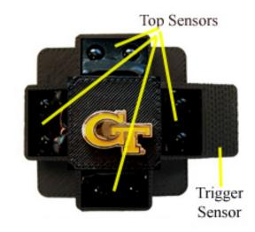
Figure 1. The Gesture Watch prototype with four sensors on the top of the device and a fifth placed horizontally to act the trigger for gesture recognition.
