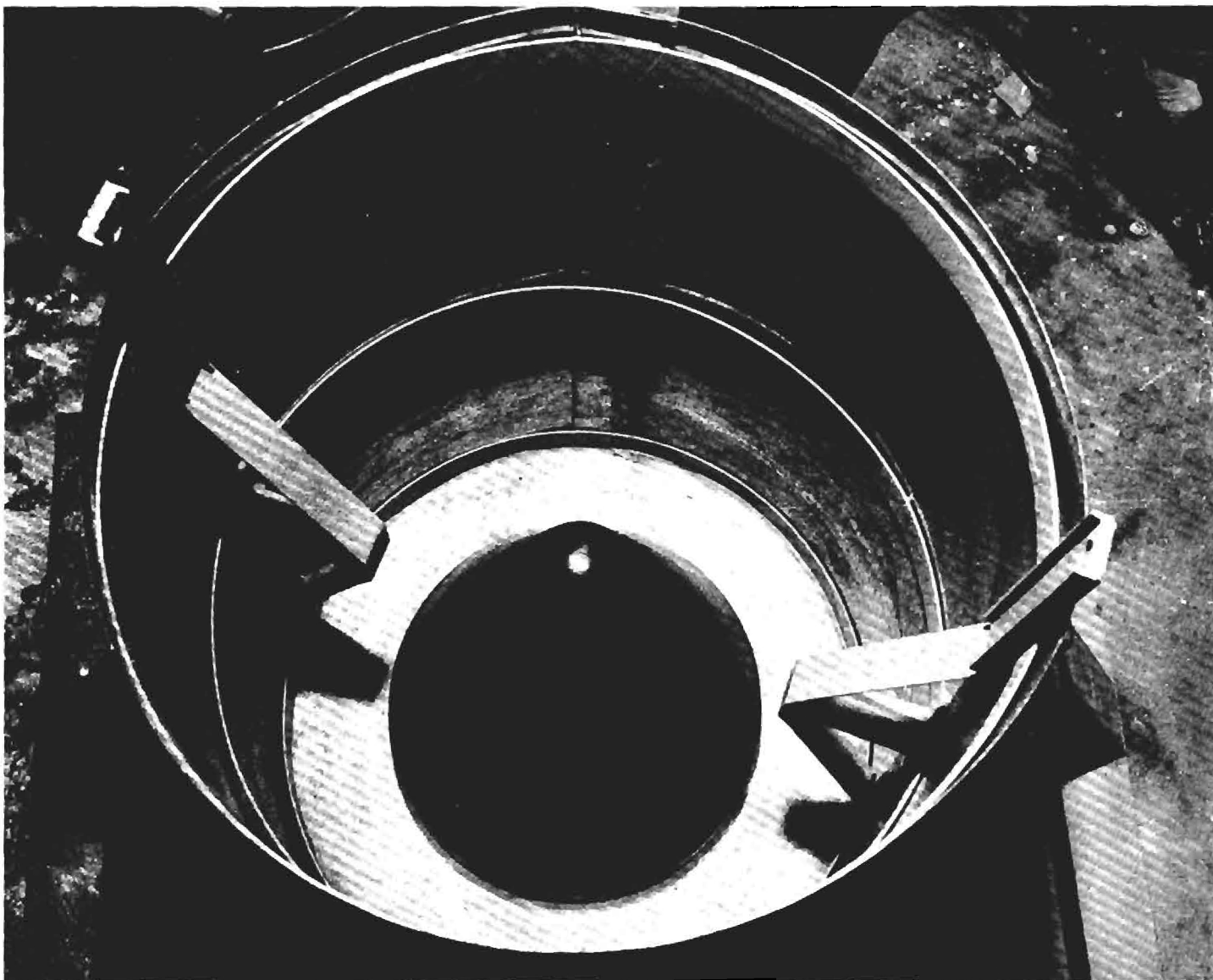
Figure 12. Head-on View of Nose Cone Model, Mold Frame, and Sheet Metal Band Previous to Casting Plaster Mold.
