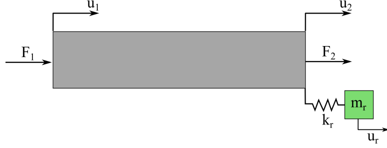
Figure 4.7: Example of a unit cell for a rod with periodically applied local resonators.
