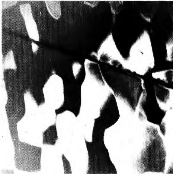
Fig. 2. Dark field image with a superlattice reflection showing APT's and APB's in \text{Ni}_4\text{Mo} after 400 minutes stress-free ordering at 700^\circ\text{C} (50,000X).
