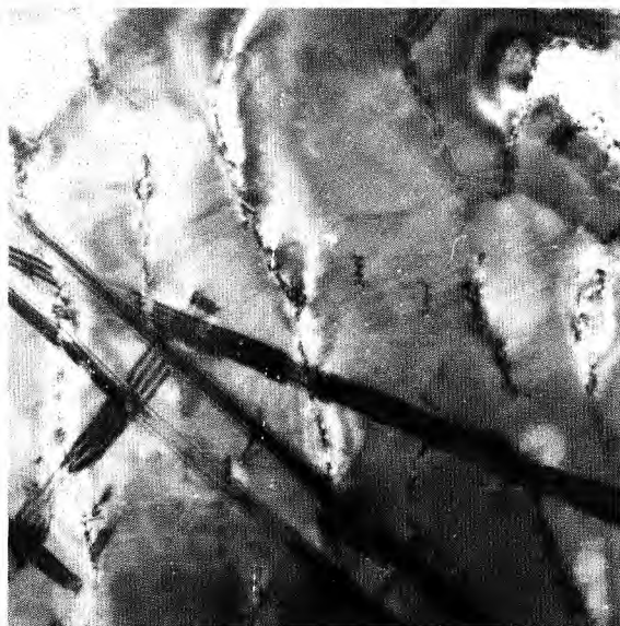
Fig. 5. Bright field electron micrograph of Ni 4 Mo stress-free ordered for 1000 minutes at 700°C [011] orientation showing low angle boundaries (40,000X).
