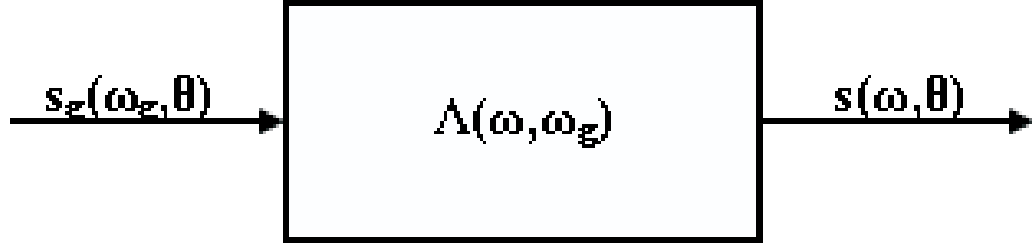
Figure 4.6. Block diagram of linear shift-varying system for generating slant-plane CSAR signal from ground-plane CSAR signal.
