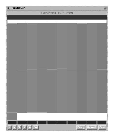
Figure 3: This blocks view is from part way through the sorting program. The first block of elements on average has small values but it still has at leat one very large value.
