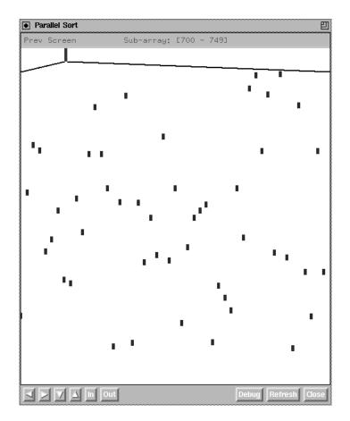
Figure 5: The view transforms its presentation when a small enough set of elements are to be shown in the display. Here, a traditional algorithm animation scatter plot sorting presentation is used where the x-dimension corresponds to position in the array, and y-dimension encodes the relative value of an element (smallest at bottom and biggest at top).
