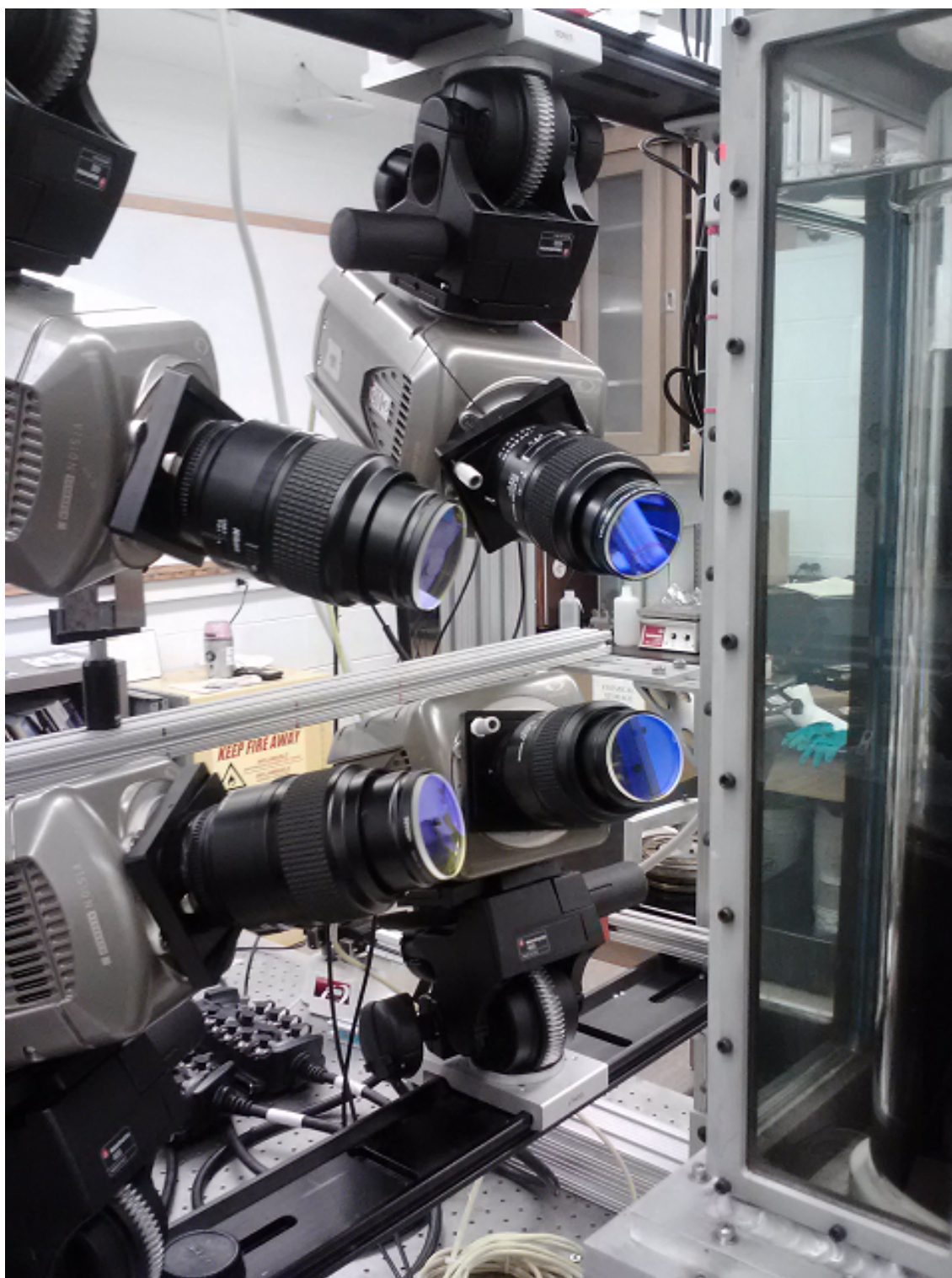
Figure 6.1: Phantom v210 cameras in the standard “cross” configuration. The cameras are equipped with 105 mm Nikon Micro lenses, LaVision Scheimpflug mounts, and Edmund Optics 550 nm long-pass filters.
