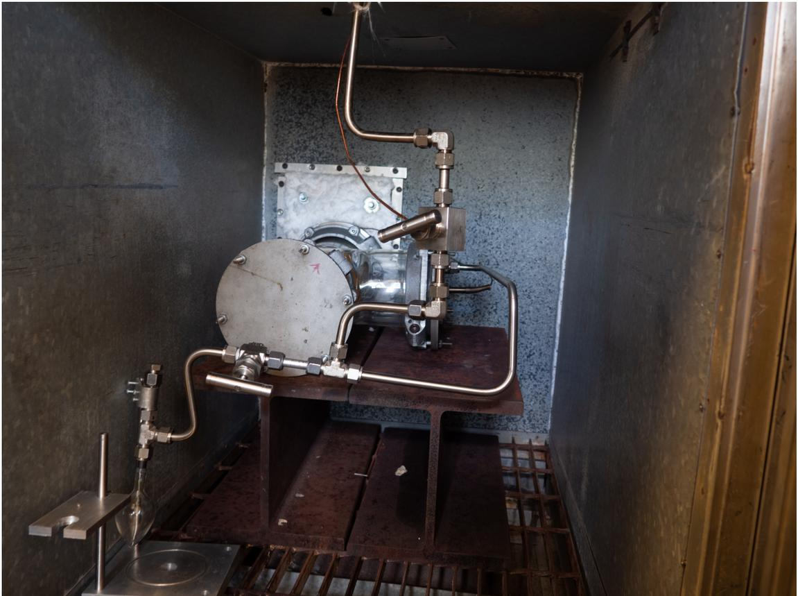
Figure 2.4: Pressure vessel and piping within the temperature chamber
