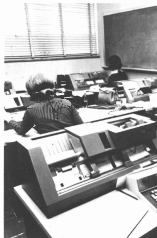
TOP LEFT: Remote terminal device, similar to a teletype machine, feeds programs directly into the computer. ABOVE: Key punch operators produce cards used in programming the computers.
