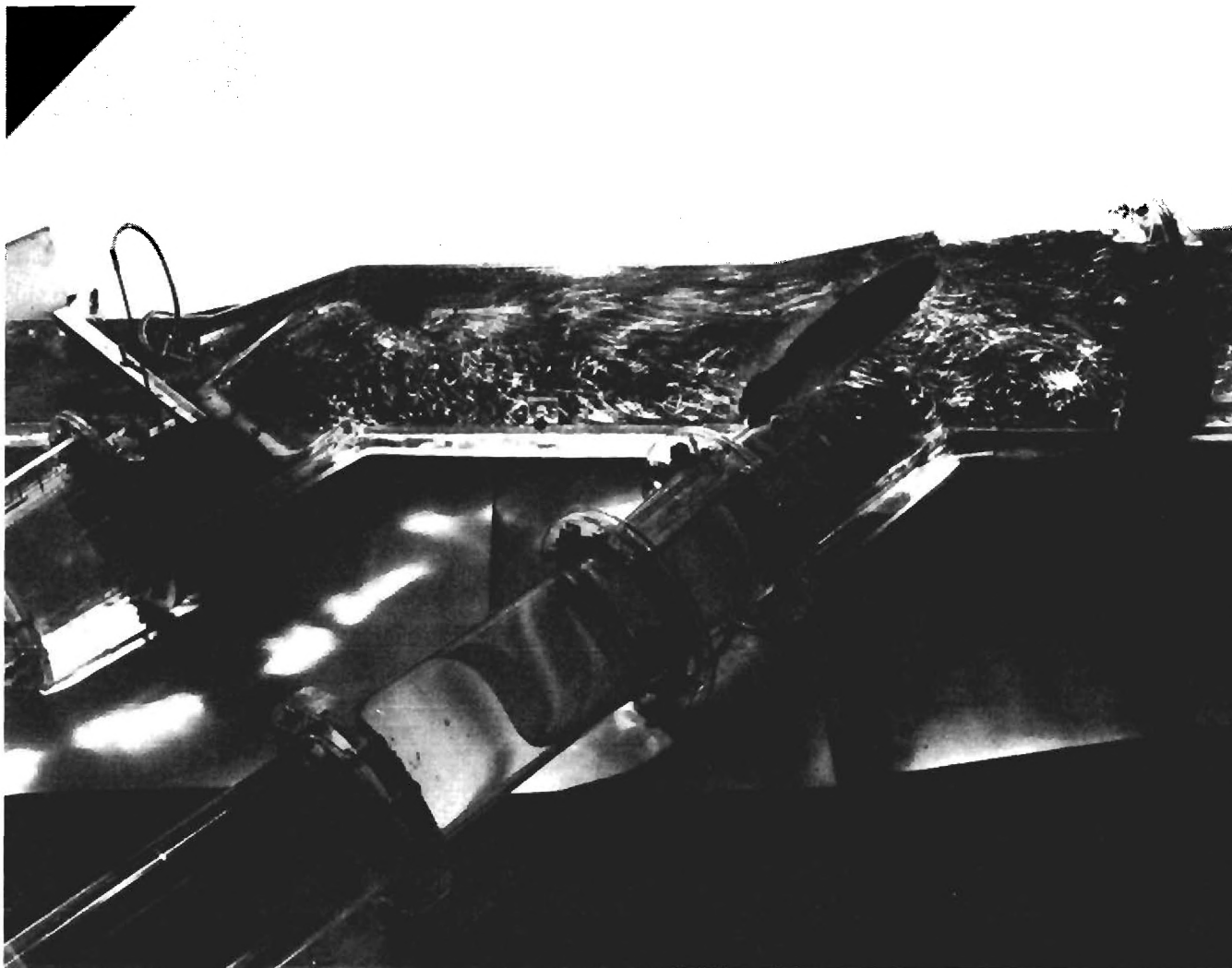
Exhibit 27. View of Tuft and Air Bubble Patterns in Trunk of Modified Scheme B-1 for Unit 1 Pumping.
