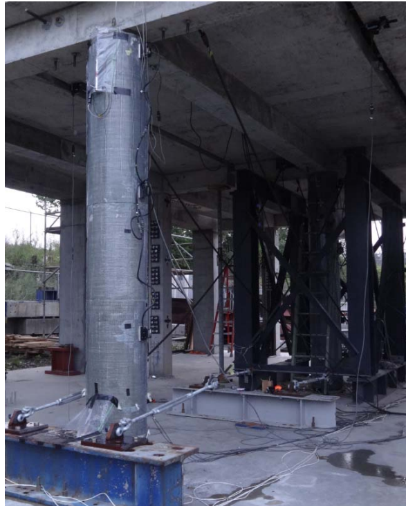
Figure 3.1. Full-scale, two-story two-bay non-ductile RC test frames: (a) four identical full-scale test frames; (b) FRP jacketed column in retrofitted test frame
