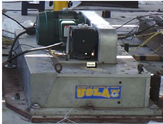
Figure 3.3. Mobile shakers: (a) hydraulic linear shaker; (b) portable eccentric mass shaker
