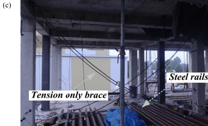
Figure 3.4. Additional test setup for collapse prevention: (a) schematic view of safety equipment; (b) first story; (c) second story
