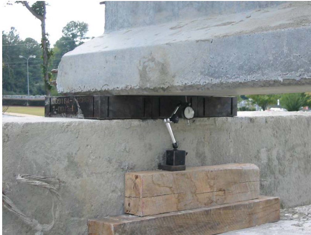
Figure 8.6 Dial gage measuring end support deflection
