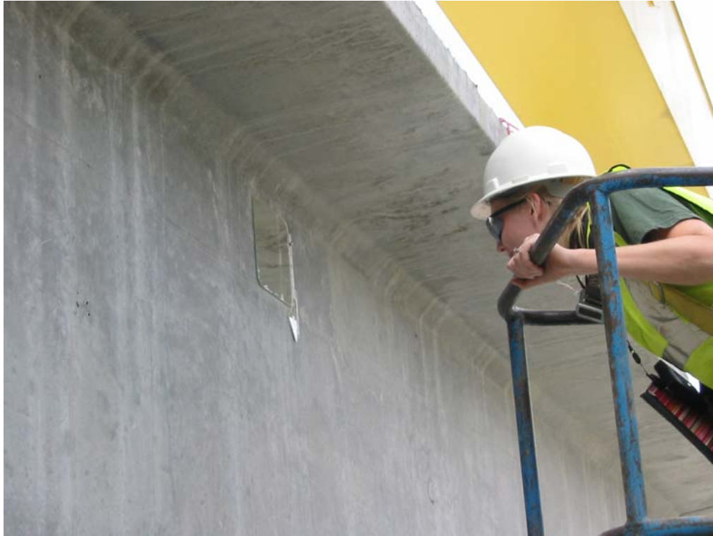
Figure 3.15 Researcher Jennifer Dunbeck reading taut wire system
