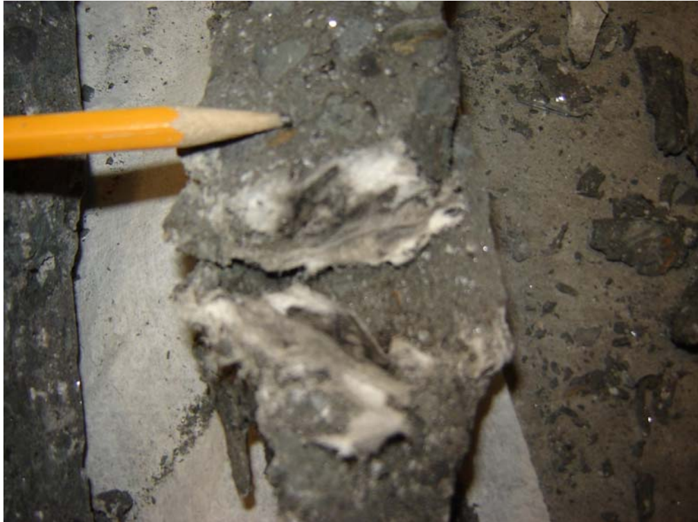
Figure 9.5 Large piece of bag woven into specimen 2-5-4-3
