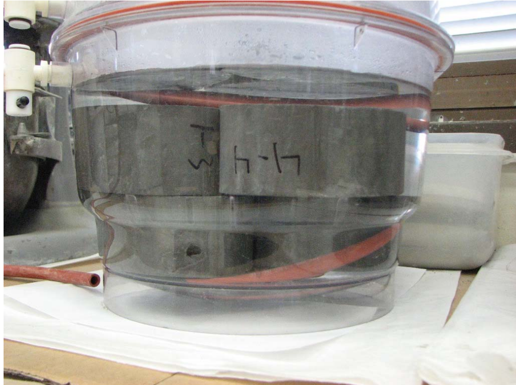
Figure 5.9 Concrete specimens soaking in vacuum desiccator
