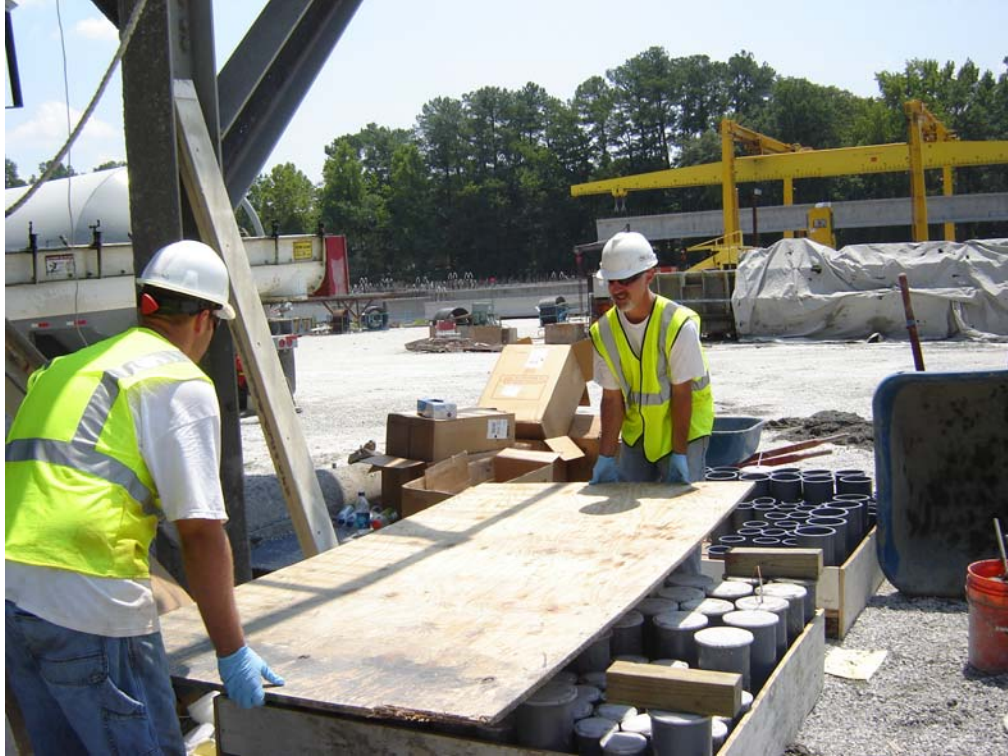
Figure 4.9 Researchers cover concrete specimens with plywood for shade
