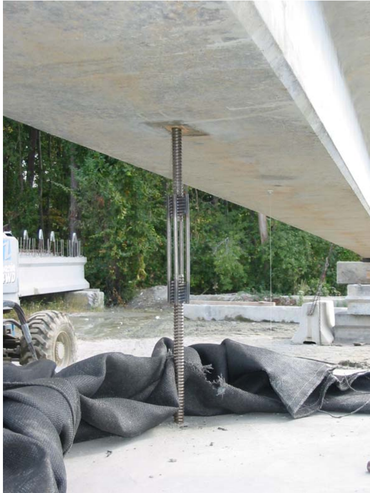
Figure 8.10 Coupler connecting load onto girder
