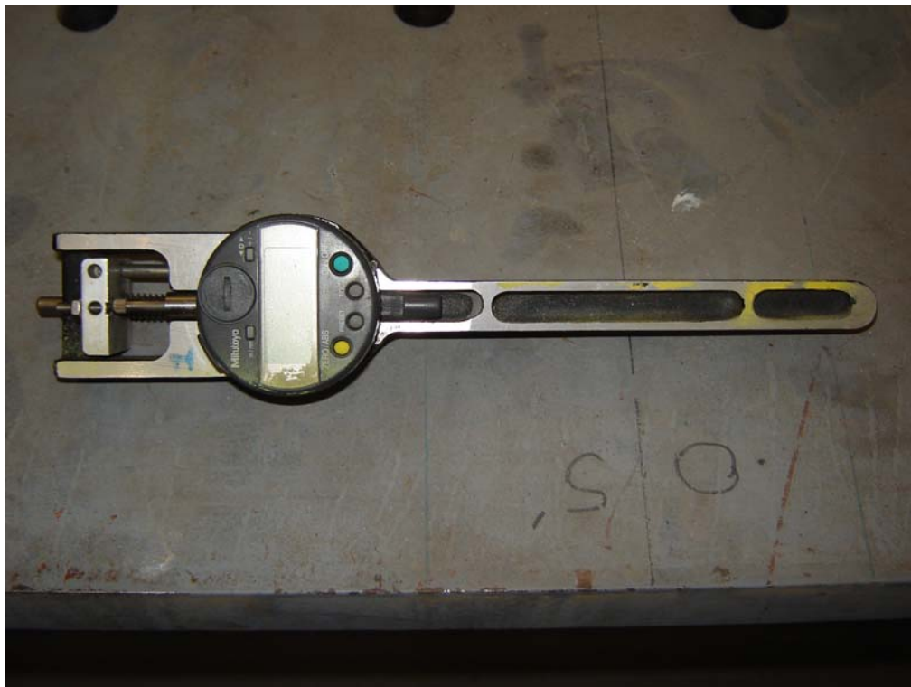
Figure 6.3 DEMEC gage used for this research
