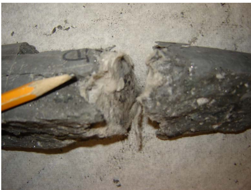
Figure 9.3 Large piece of bag is folded inside 4"x 8" cylinder 3-1-4-3
