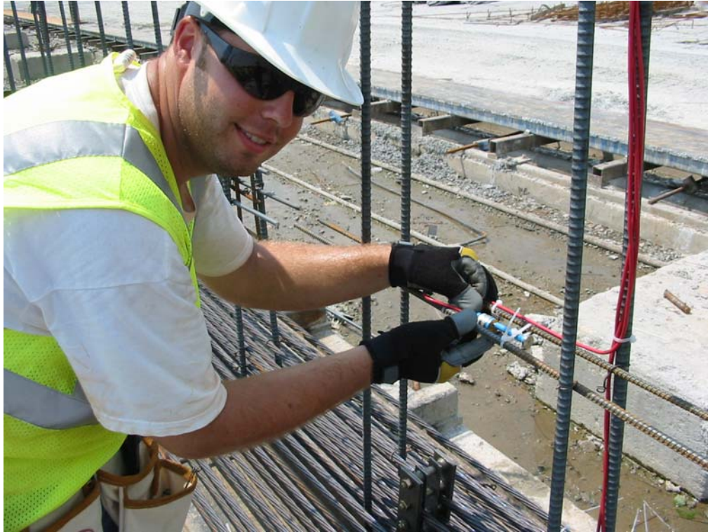
Figure 3.6 Researcher Brett Holland securing VWSG at midheight of girder
