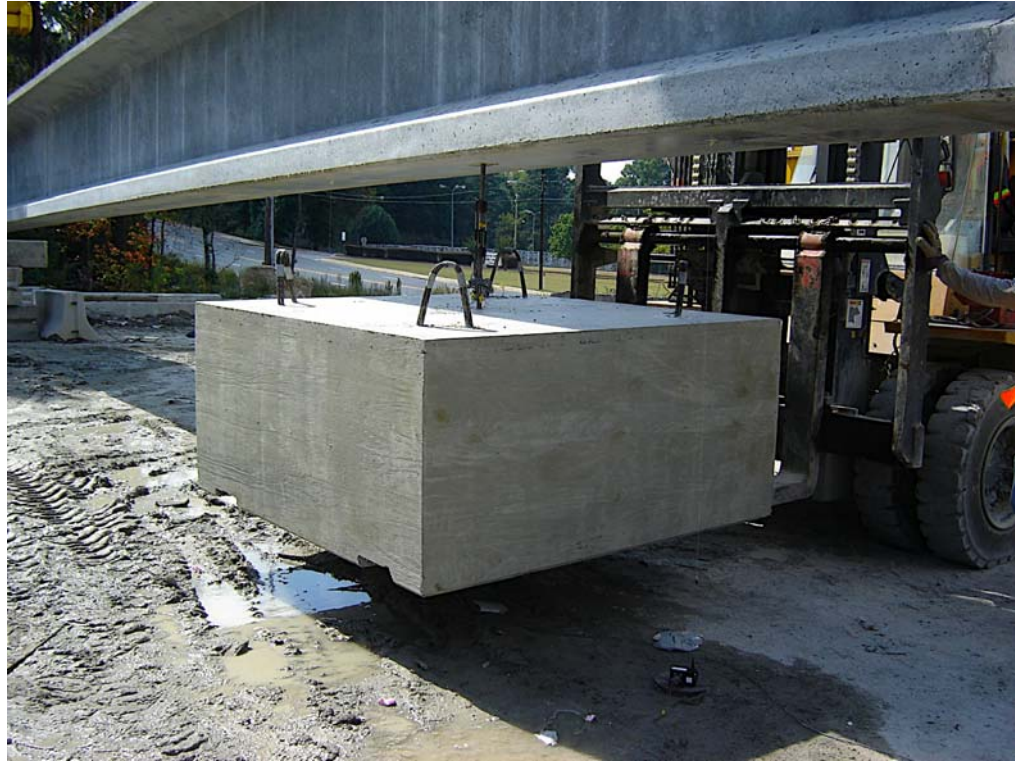
Figure 8.8 Reinforced concrete block used to load girders
