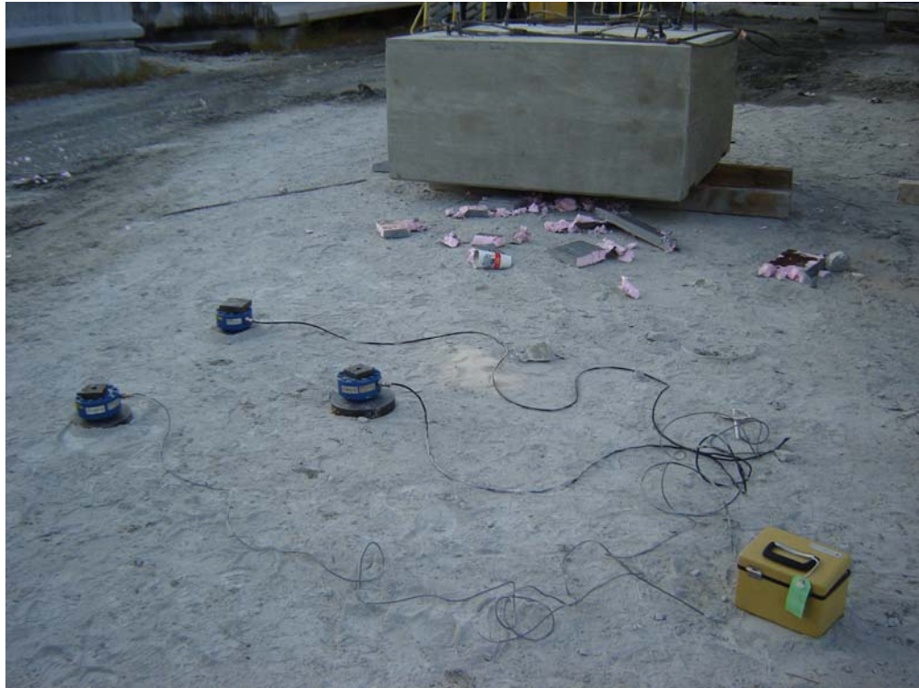
Figure 8.7 Three load cells and strain indicator box used to weigh the load block
