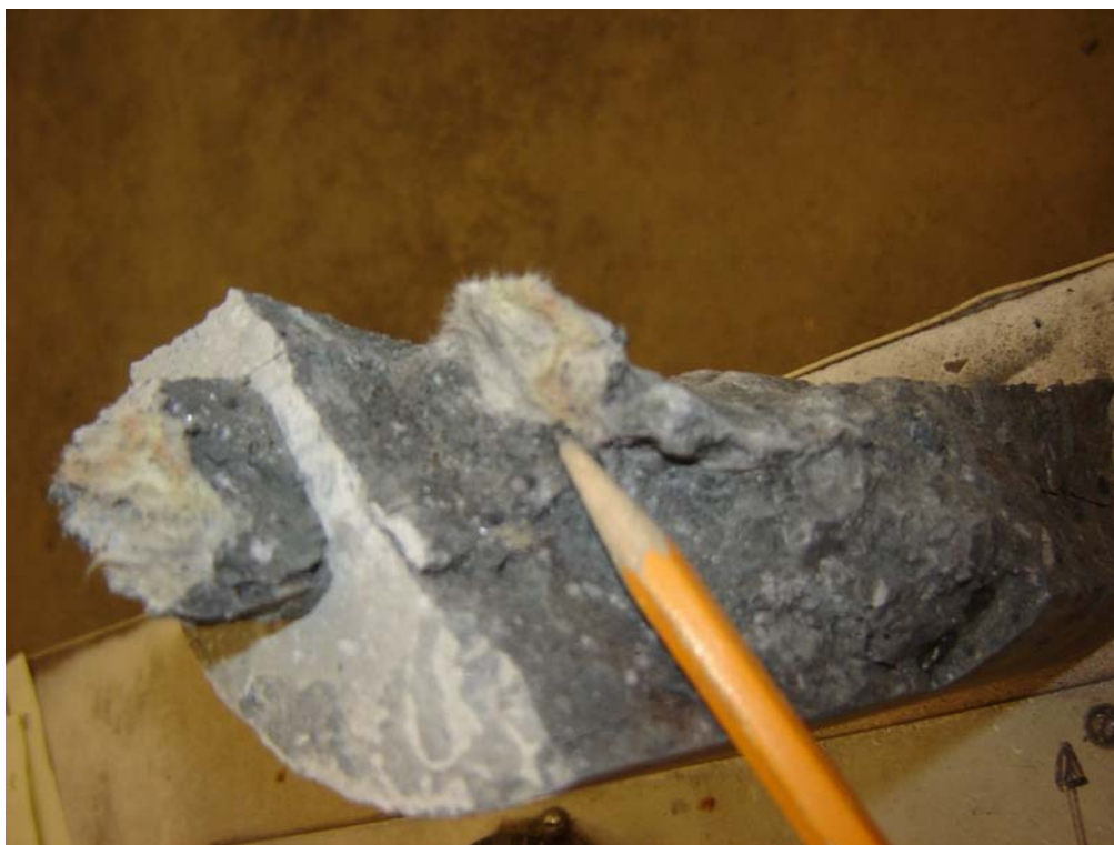
Figure 9.2 Medium piece of bag in cylinder 2-5-4-2
