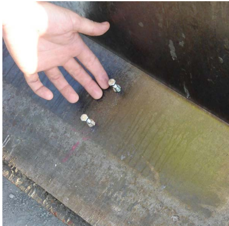
Figure 3.17 Embedments in bottom flange of steel forms for attachment of angles
