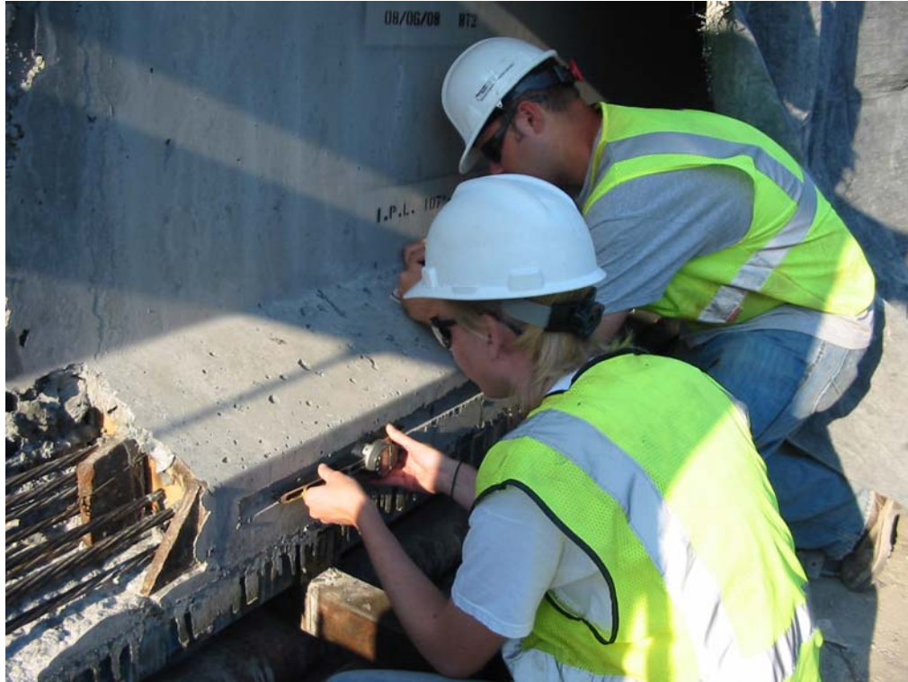
Figure 6.4 Researchers Jennifer Dunbeck and Brett Holland taking DEMEC readings
