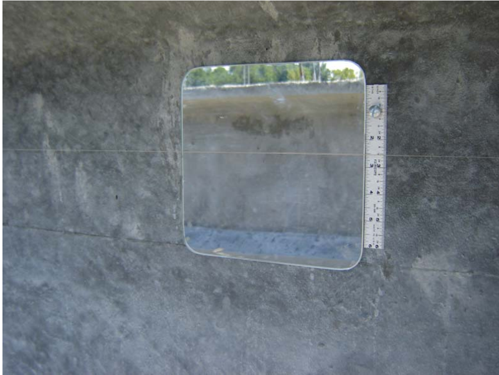
Figure 3.19 Primary ruler with mirror adjacent and taut wire running across
