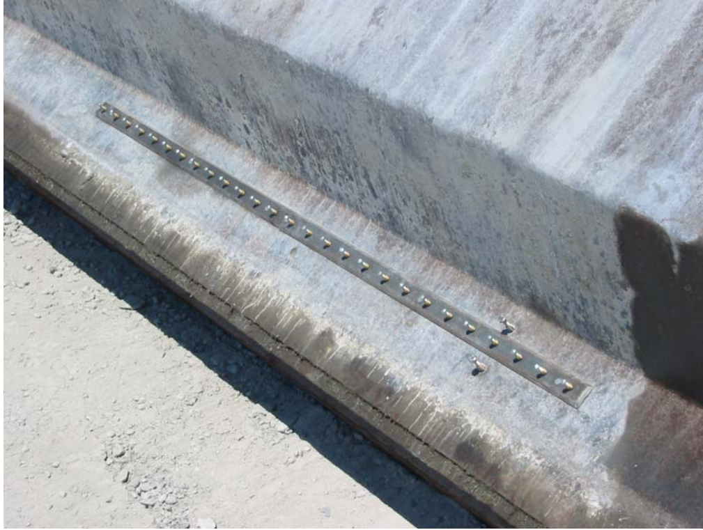
Figure 3.20 Transfer length embedments attached to forms
