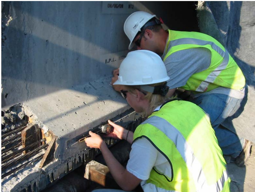
Figure 3.21 Researchers taking DEMEC gage readings on girder end before cut-down
