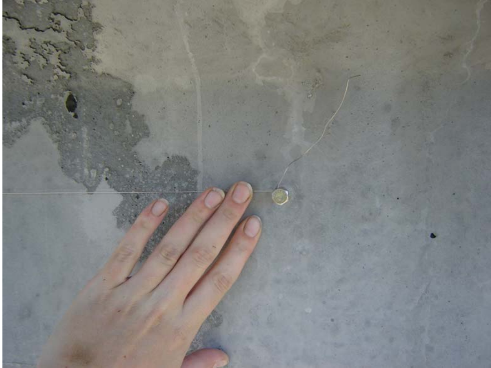
Figure 3.18 Bolt screwed into embedment in girder face with taut wire tied around it
