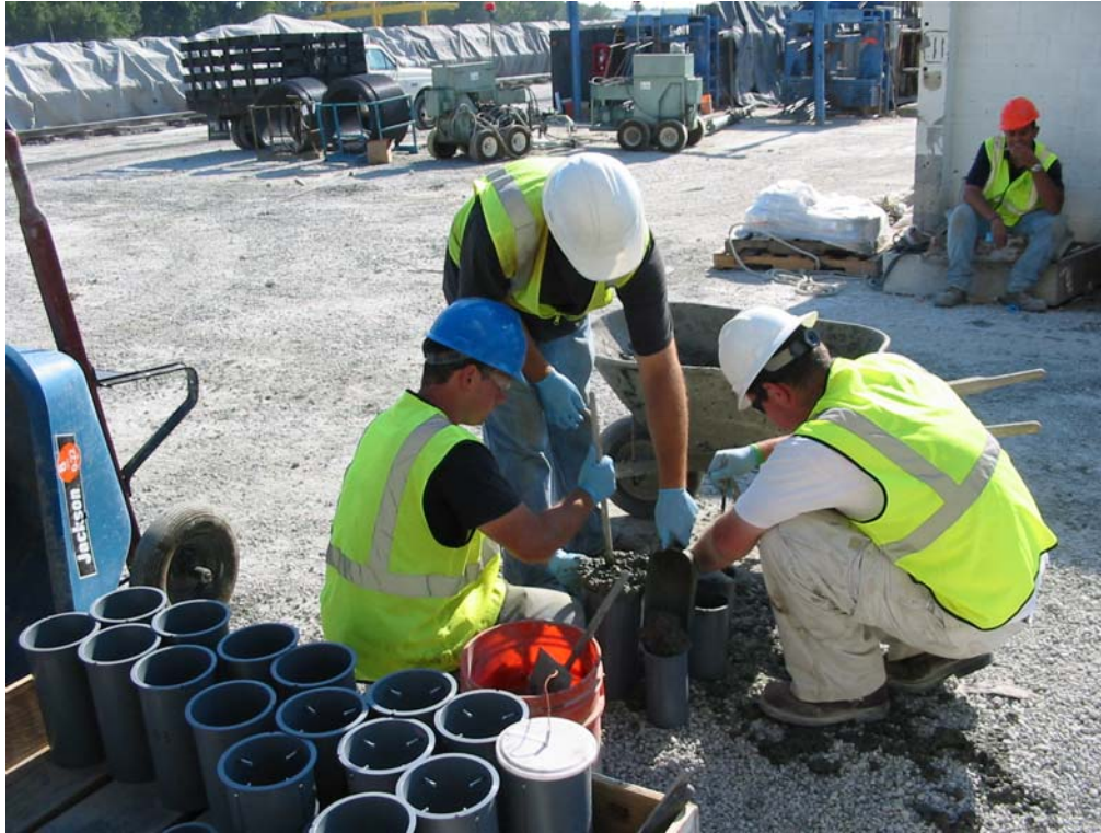
Figure 4.8 Georgia Tech GRAs construct concrete cylinder specimens
