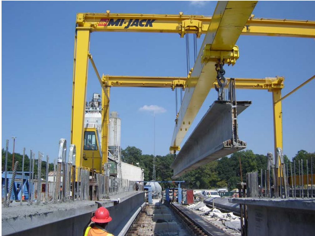
Figure 4.19 Straddle-lift picks girder up off construction bed
