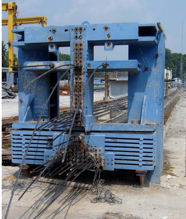
Figure 3.9 Dead end abutment with prestressing strands and load cells in place
