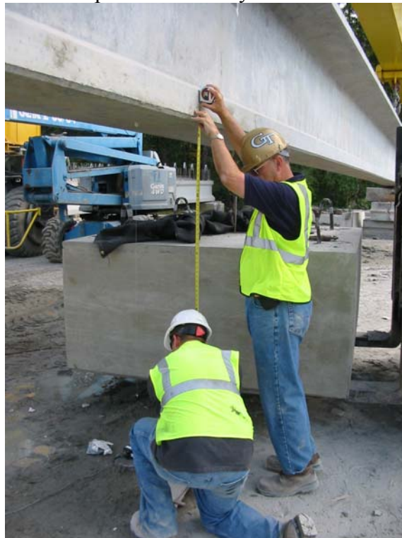
Figure 8.11 Researcher reading taut wire measurement; Dashed line is used to depict wire which is barely visible in photo. Accuracy 1/32 inch.
