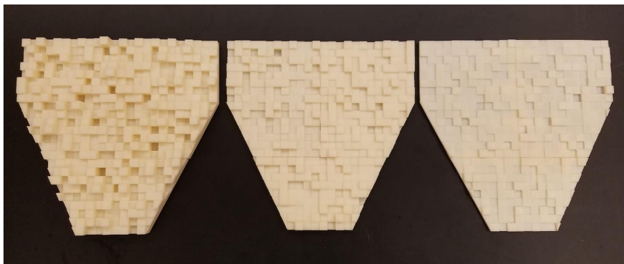
Figure 1. The three terrain bases after printing and assembly utilized in this experiment. From left to right, the standard deviations of their gaussian distributions are 0.5cm, 0.2cm, and 0.1cm respectively.
