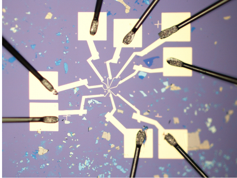
Figure A.7: Optical micrograph of a Hall bar patterned onto a graphene flake after the developing the PMMA.
