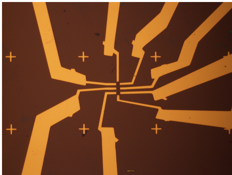
Figure A.6: Optical micrograph of a graphene device after wire bonding to the gold contact pads.
