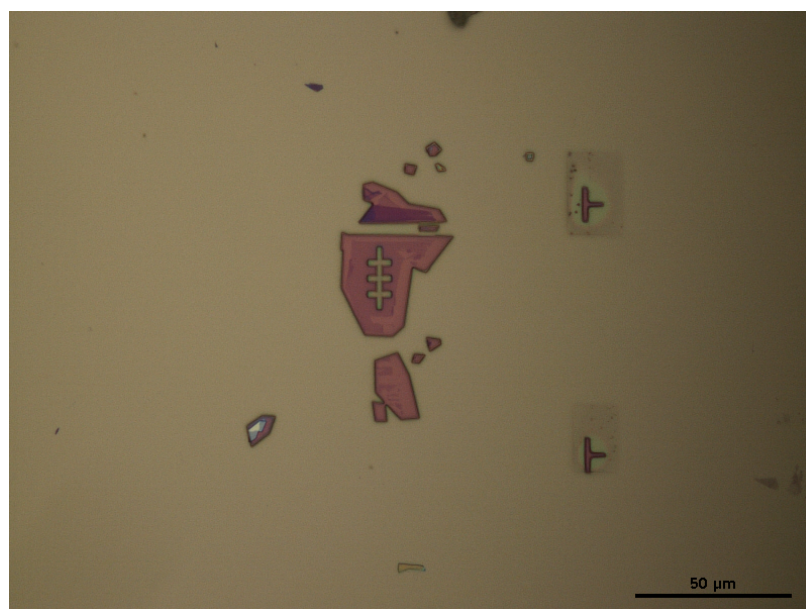
Figure A.3: Optical micrograph of a Hall bar patterned onto a graphene flake after the plasma etch of exposed graphene.
