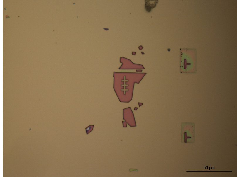
Figure A.4: Optical micrograph of a graphene/gold contact lines after developing the PMMA.
