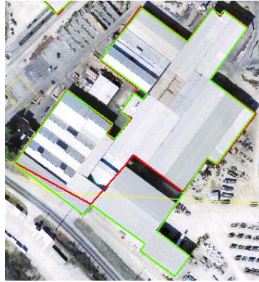
Figure 129 – (green) building footprint as digitized on a full image (red) building footprint as digitized on a parcel sized image (yellow) parcel boundary
