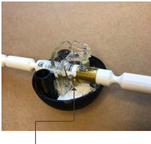
Main locking piece as seen when the sphere is taken apart. This locks the sphere into place on the rod.
