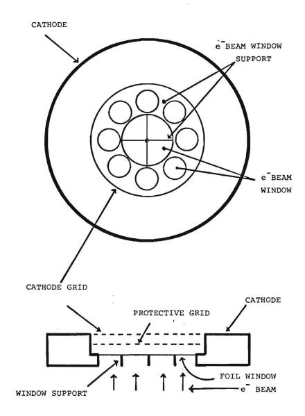
Figure 5. Front and Side View of Cathode and Electron Window Assembly.
