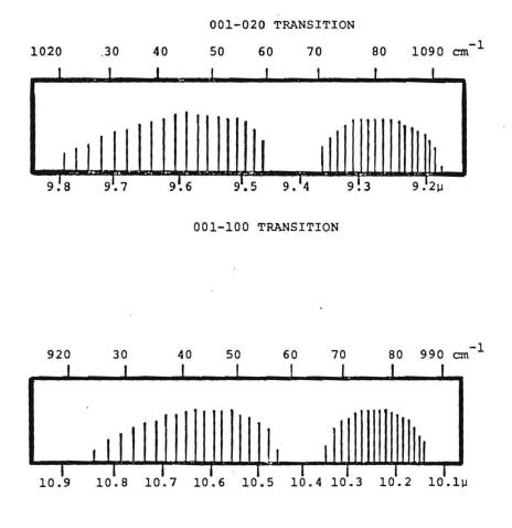
Figure 13.  $CO_2$  Laser Lines Used to Study  $NF_3$ ,  $C_3F_8$ and  $CO_2$ .
