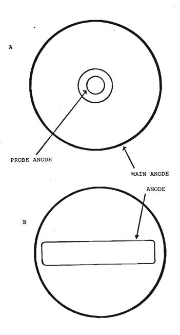
Figure 6. The anode configuration shown in (A) above was used for the majority of this study, while (B) was used to improve the sensitivity for the final HCl and HCN measurements.
