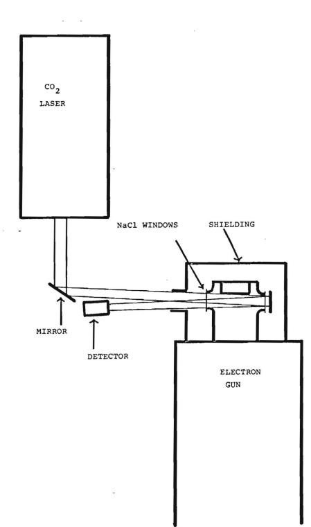
Figure 8. The Experimental Configuration Used to Study  $NF_3$ ,  $C_3F_8$ , and  $CO_2$ .
