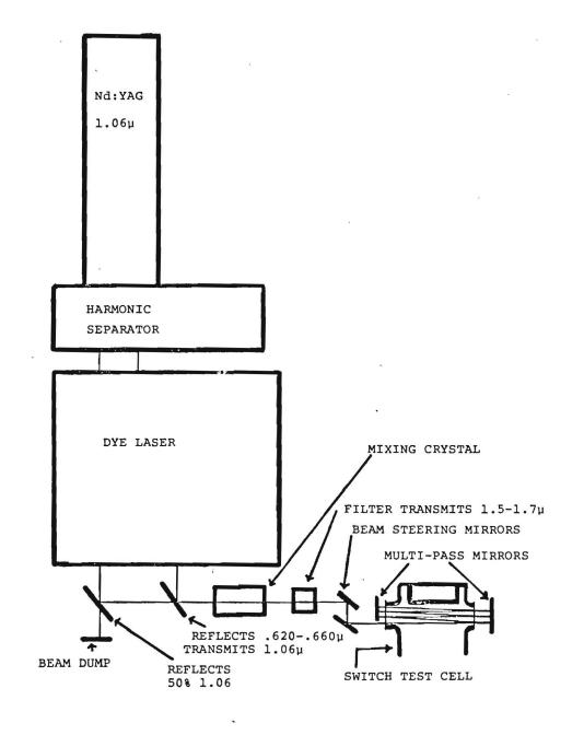
Figure 10. Frequency Mixing Technique Used for the Excitation of HCl and HCN.
