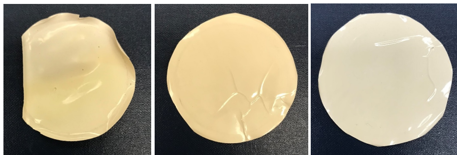
Figure 6. Dry membranes crosslinked with a) ethylenediamine, b) 1,6-hexanediamine, and c) para-xylylenediamine
