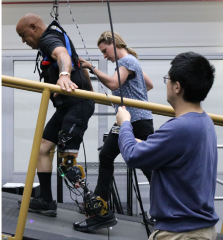
Figure 5.10: Experimental protocol using Open Source Leg (OSL) on ramp ascent. The powered device scales knee assistance as a function of slope angle throughout early stance.
