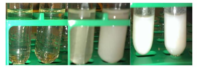
Figure 7.17: Picture of reactive-crystallization Run 4 and 5 when reaction started (left), after seeding (center), and after 6 hours (right).
