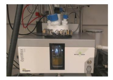
Figure 7.2: 250 mL reactive crystallization set up.
