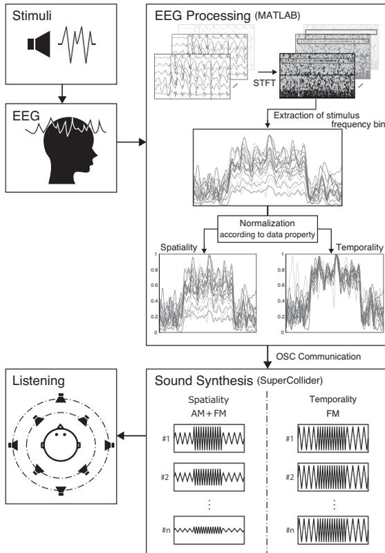
Figure 1: The framework of proposed SSR sonification method.
