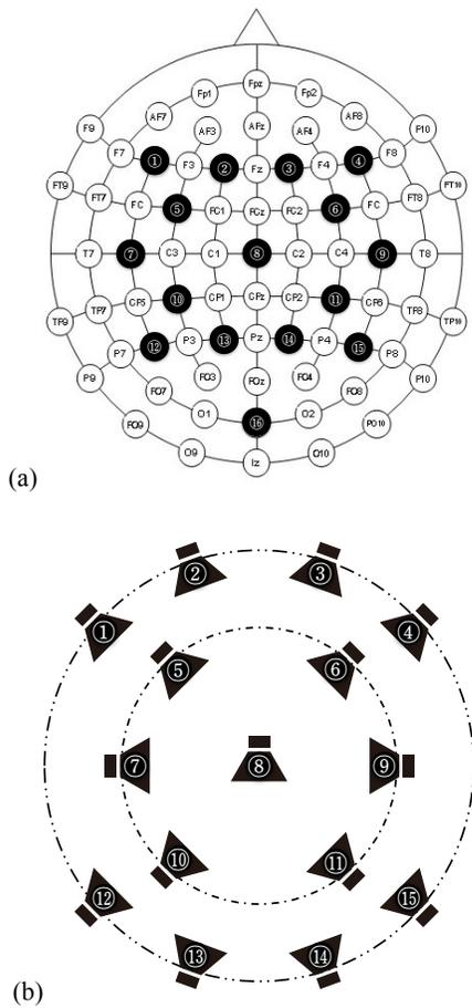
Figure 2: The association between loudspeakers and EEG measurement positions. (a) shows 16 EEG measurement positions. (b) shows the arrangement of 15 loudspeakers associated with EEG measurement position (the outer circle corresponds the middle height, and the inner circle and the center speaker is at the ceiling height.)
