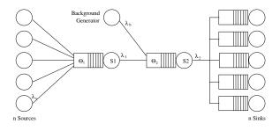
Figure 5: Simple Two-Stage Topology
