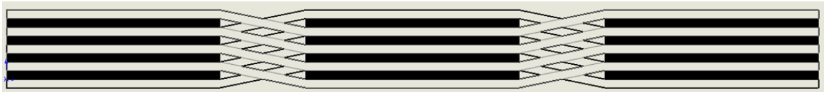
Figure 48: Cross-section of 2D plain weave fabric geometry. Warp tapes (foreground and background) run from left to right. Weft tapes come out of page and are shaded black.
