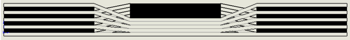
Figure 49: Cross-section of plain weave fabric geometry with single 3D interlace point (middle). Warp tapes (foreground and background) run from left to right. Weft tapes come out of page and are shaded black.
