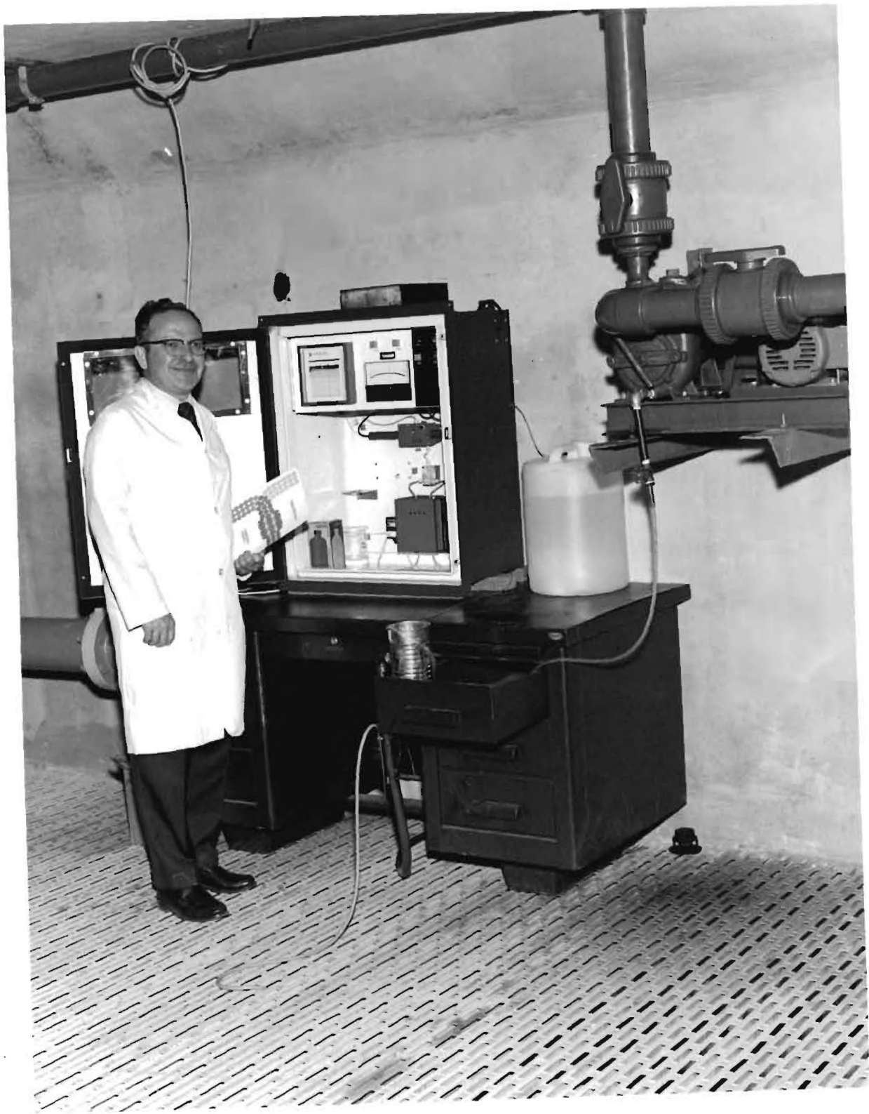
Figure 8. Series 1000 Fluoride Monitor of Orion Research installed at Flint River Plant, Atlanta, Georgia.
