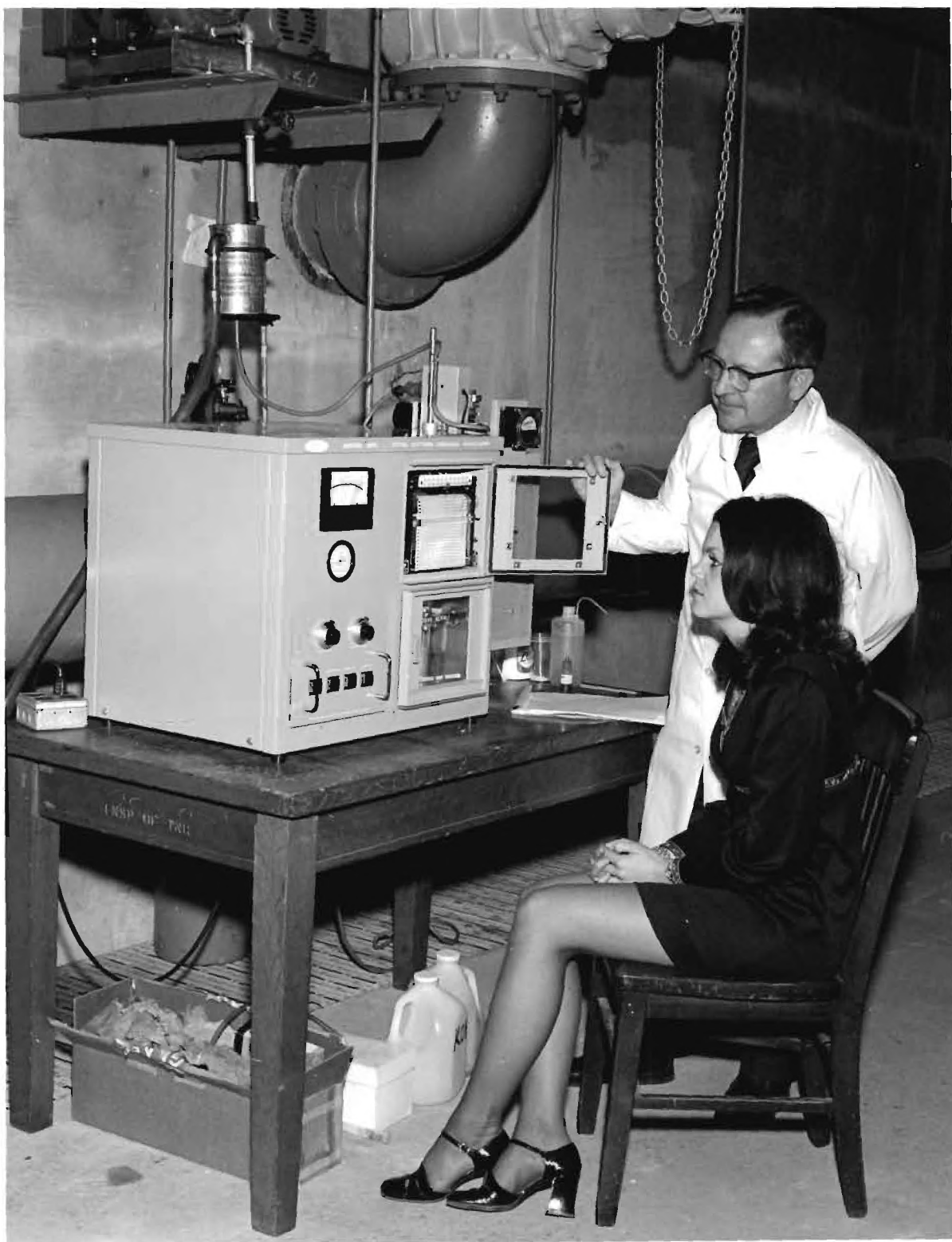
Figure 5. Total Oxygen Demand Analyzer of Ionics, Inc. installed at Flint River Plant, Atlanta, Georgia.
