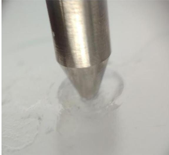
**Figure 6: Close-up of the GK pin embedded into the Castn'Craft liquid acrylic surrounded by Lucite.**
