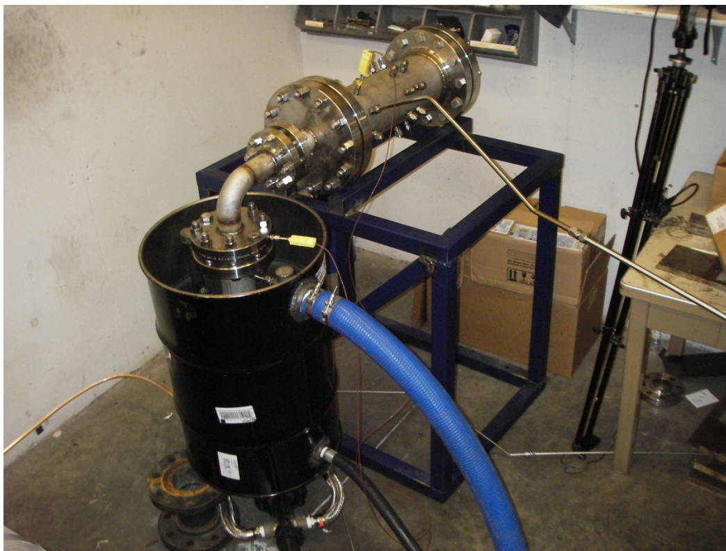
Figure 22: Vitiator in its drum, and fuel cell vessel.
