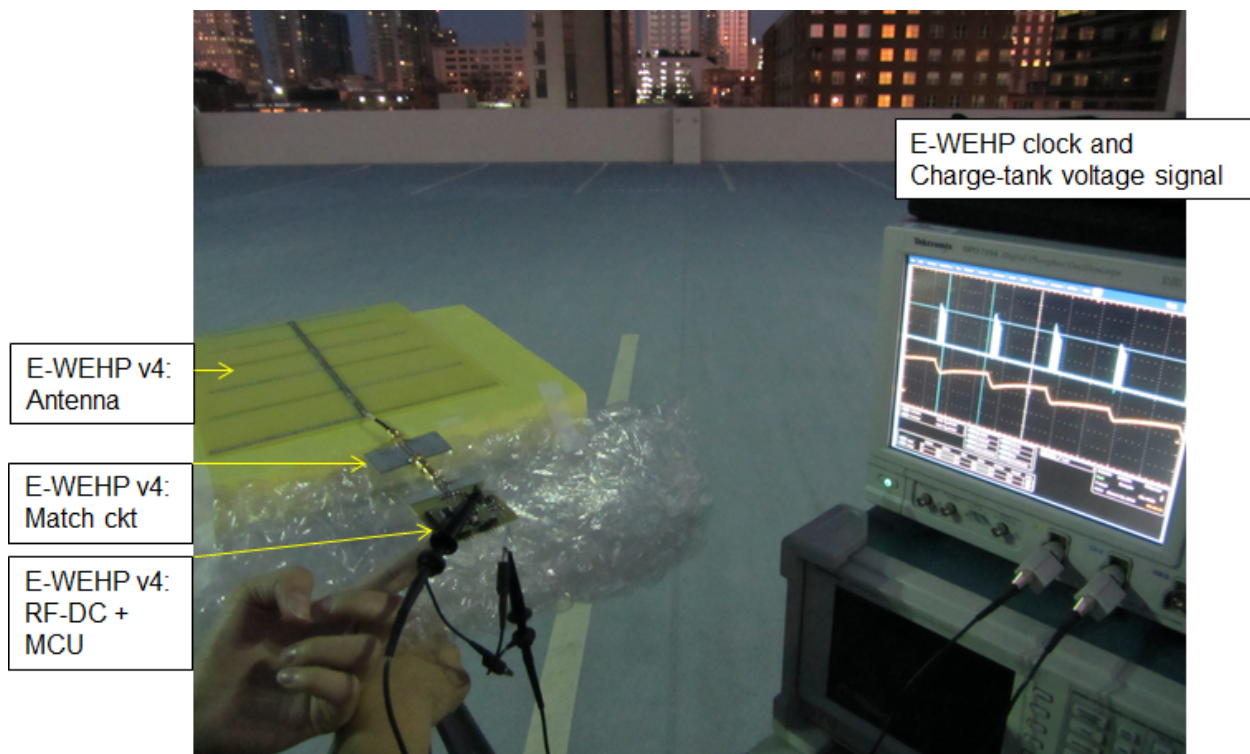
Figure 100. Self-sustaining E-WEHP embedded operation powered from power in wireless CBS and IND TV signals with combined channel power of -13.92dBm in Midtown Atlanta.
