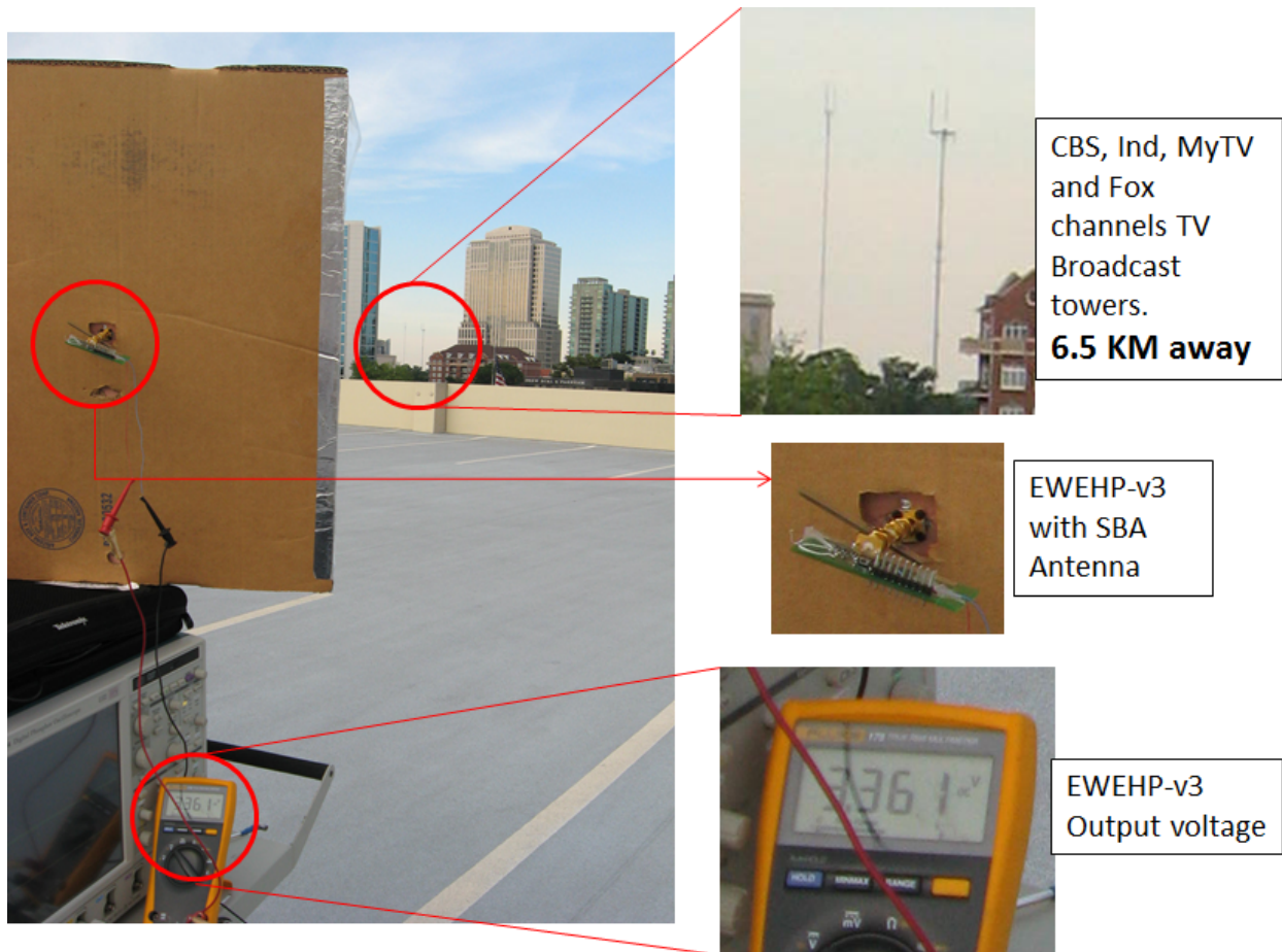
Figure 89. Field measurement with E-WEHP v3 prototype and SBA antenna harvesting wireless energy from wireless digital TV signals broadcasted from atop TV towers 6.0 km away in Midtown Atlanta.
