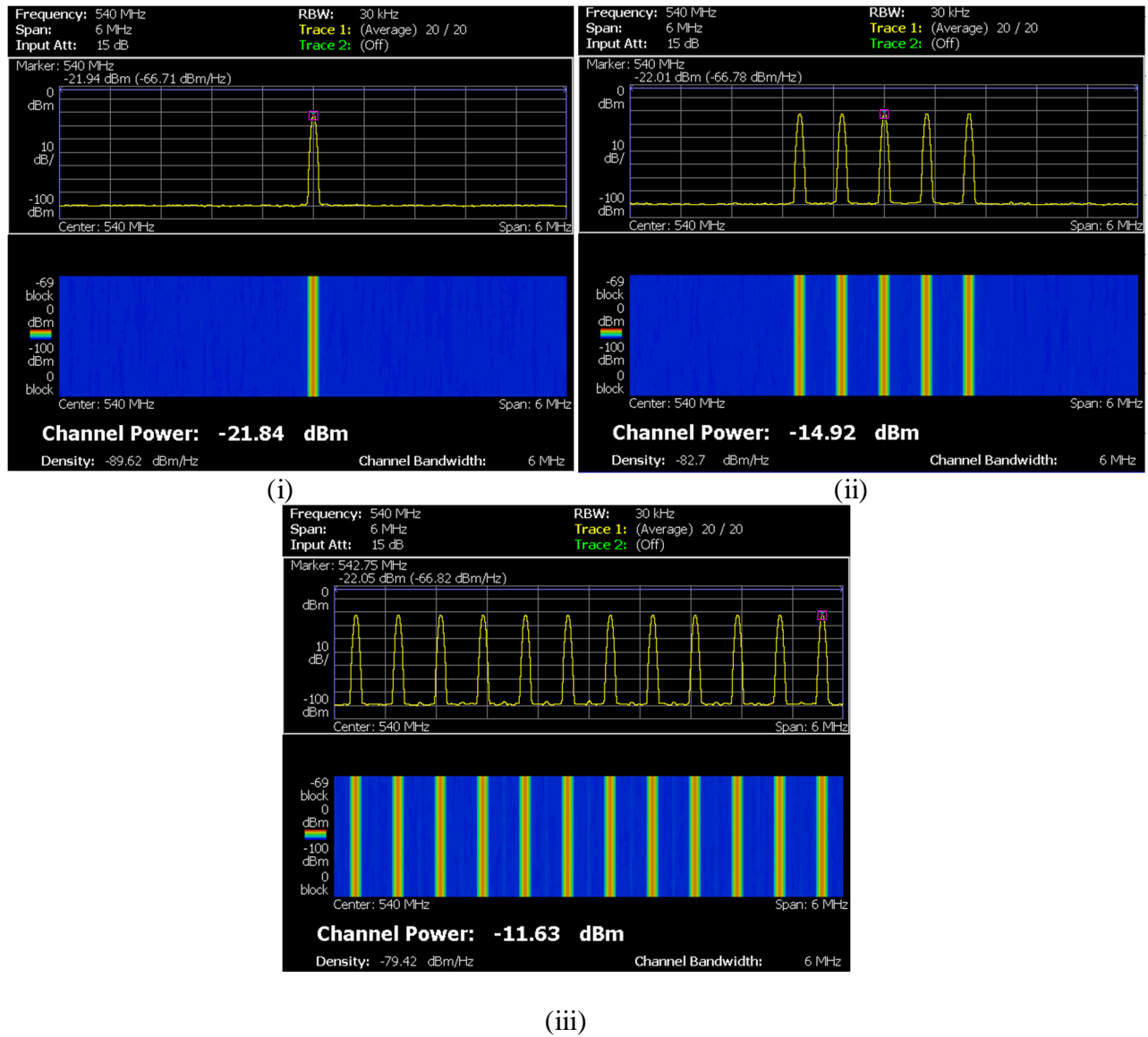
Figure 77. Multi-tone signal inputs generated by Rohde and Schwarz SMJ100A Vector signal generator to test multi-tone response of E-WEHP RF-DC circuit.
