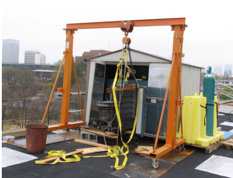
Figure 4. The Grieve oven (AB-650) and the Custom Hays Fabrication and Welding Pressure Vessel
