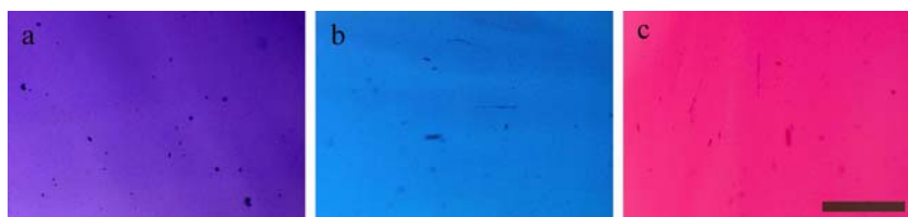
Figure 6.11. Optical micrographs of drawn PVA-gold nanocomposites with ca 4 wt % gold NPs mixture and draw ratio 4. a) unpolarized, b) polarization direction parallel to the drawing direction and c) polarization direction perpendicular to the drawing direction. Scale bar is 50 \mu m.
