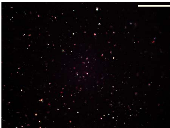
Figure 4.11. Gold NRs flocculation observed under the microscope with crossed polarizers. The scale bar is 100 \mu m.
