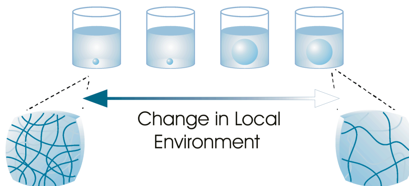
Figure 1.1 Schematic representing the volume phase transition of a responsive hydrogel.
