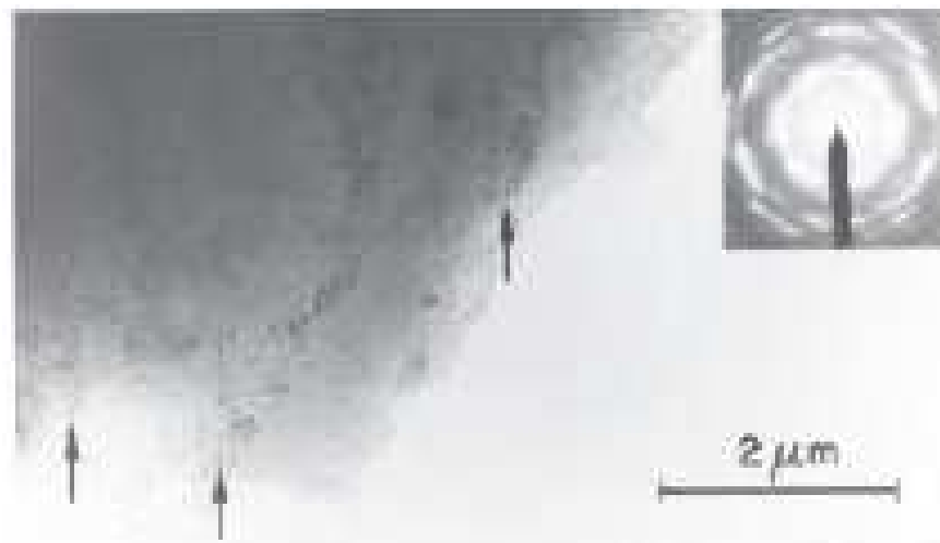
Figure 2.11: TEM bright field image of AIRu powder after 10 minutes of milling.
