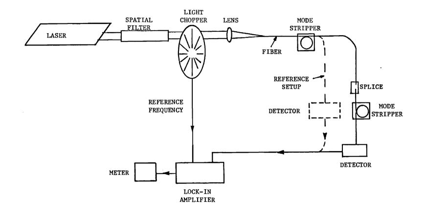
Figure 3 - Block Diagram for Splicing Loss Experiment
