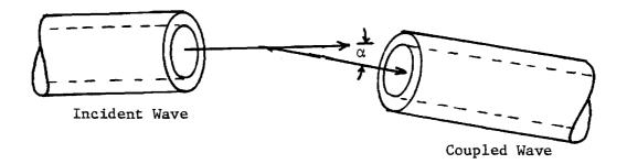
Figure 2 Experiment for Angular Splicing Losses
