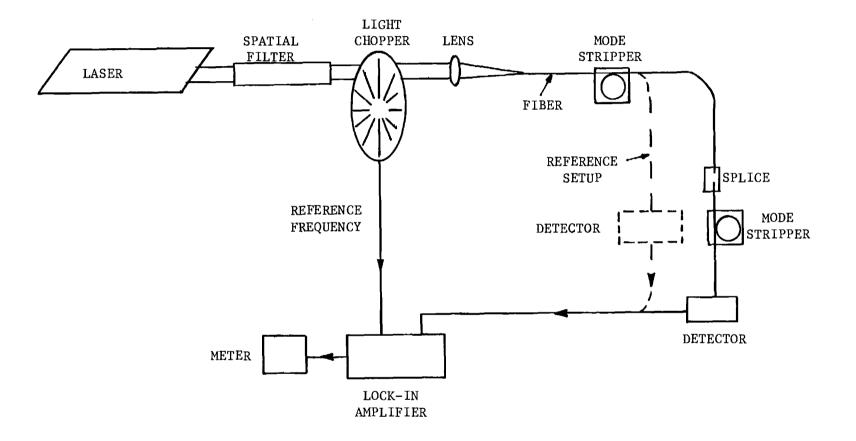
Figure 1 - Block Diagram for Splicing Loss Experiment
