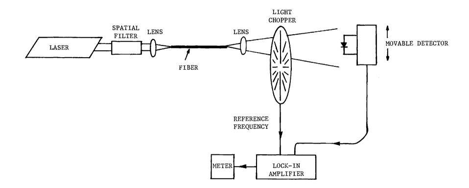
Figure 3 - Block Diagram for Index Profiling Experiment
