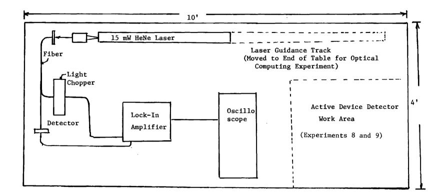
Basic Layout of Workspace Allottment on Isolated Optical Bench
