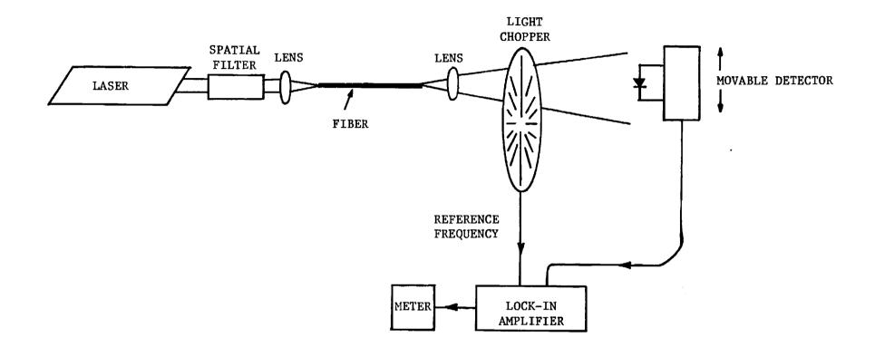
Figure 4 - Block Diagram for Index Profiling Experiment
