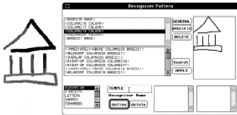
Figure 3-11. A configuration can be named and define in a search window that displays and analyzes element types and spatial relations between elements. For example, shown here a ‘temple’ is defined with a ‘roof’ immediately above row of ‘columns’ immediate above a ‘base.’
