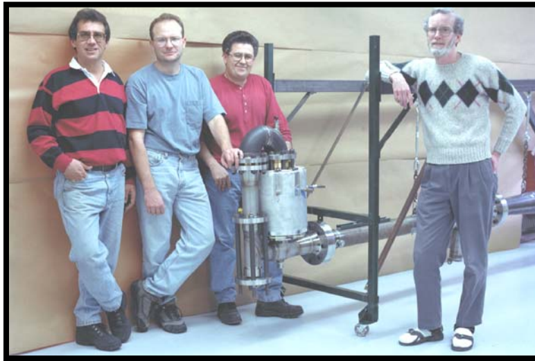
Figure 2.3: Los Alamos National Laboratory's 1kW thermoacoustic-Stirling heat engine (TASHE) [11] surrounded by its designers.
