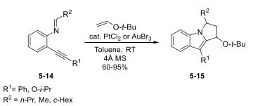
Figure 5.5: Pt(II)- or Au(III)-catalyzed [3+2] cycloaddition for 2,3-dihydro-1*H*-pyrrolo[1,2-*a*]indoles
