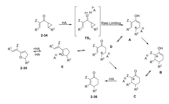
Figure 2.9: Waser's mechanism for the formal homo-Nazarov cyclization
