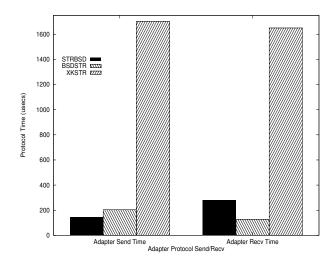
Figure 8: Adapter Protocol Timings (usecs)
