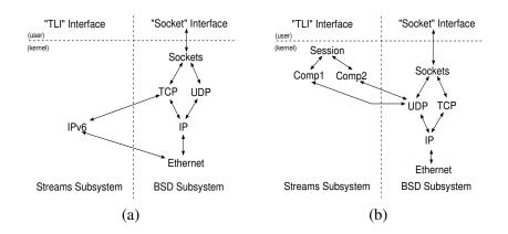
Figure 1: Multi-Subsystem Protocol Graph Examples
