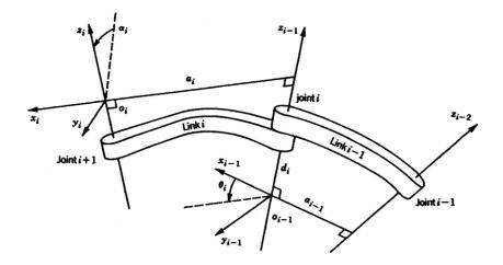
Figure 1: Frames assigned to actuators and the parameters  $\{\alpha, \theta, a, d\}$  (From [1])
