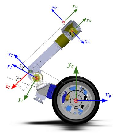
Figure 2: The base frames and the joint angles from the side view
