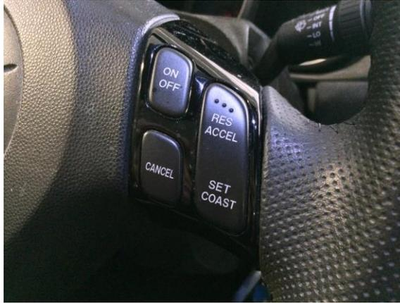
Figure 4. Example of a Steering Wheel Switch Pack
