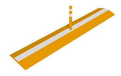
Figure 6: Illustration of the Linear Channelizing Device used in Experiment 2. These segments would be placed end-on-end to create both closure and continuity.
