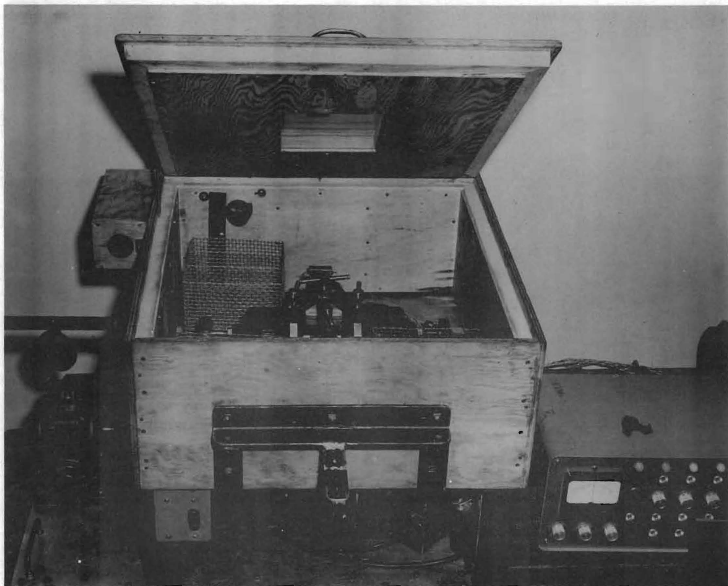
Figure 3. The Biaxial - Fabric - Tension - Testing Machine with Insulated Hood.
