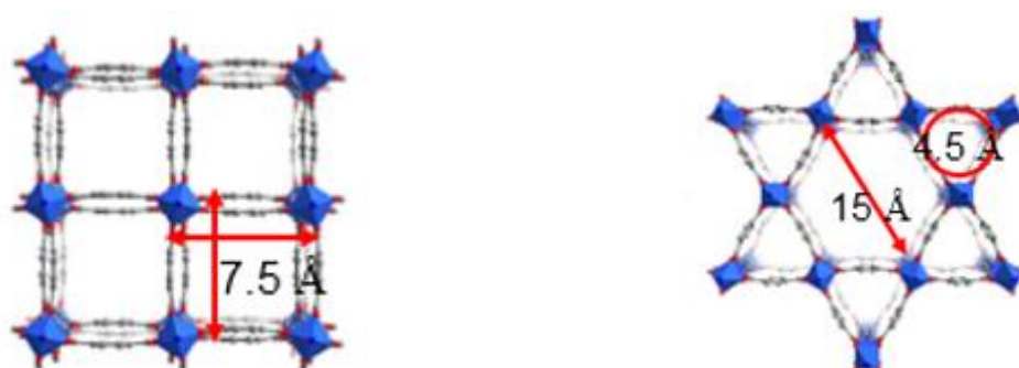
Figure D.2: Crystal structure of DMOF-1 (left) and ZnBD (right). “Reproduced from 5. Copyright 2017, Elsevier.”
