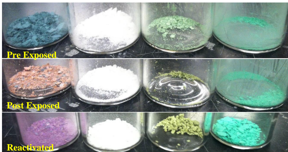
Figure E.13: Pictures of Pre Exposed, Post Exposed, and Post Exposure Reactivated Samples of M-DMOF-TM for Humid \text{SO}_2 Exposure. Samples are Co, Zn, Ni, Cu from Left to Right.
