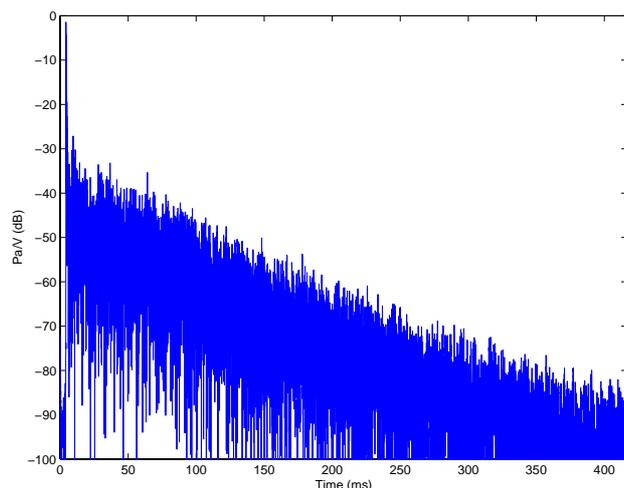
Figure 3 Measurement of a binaural room impulse response (BRIR) shown on a logarithmic scale.
