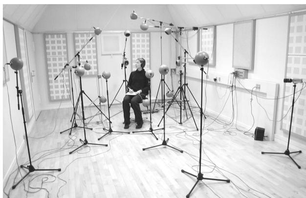
Figure 1 Set-up of loudspeakers in the listening room. Listeners were allowed to move freely while seated on the chair.
