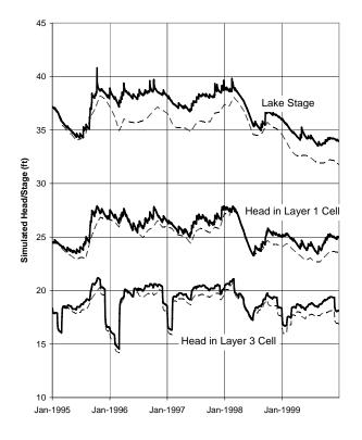
Figure 2. Simulated lake stage and groundwater head at selected model locations with the SV Package (solid lines) and without the SV Package (dashed lines).
