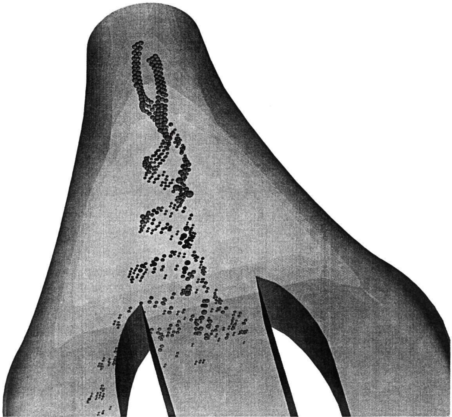
Figure 8. Bubble propagation in TVA's Norris Project draft tube. Maximum gate and partial deflector aeration conditions
