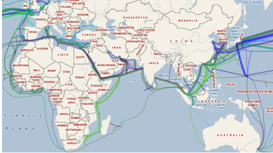
Figure 30: Undersea cables between the US and other countries. Though not shown, the cables travel across either the Atlantic or the Pacific to reach the US.
