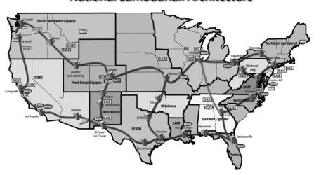
The map shows the distribution of fiber optic cable and the locations of the network's nodes. Data transmission along the network is 10 gigabits per second.
