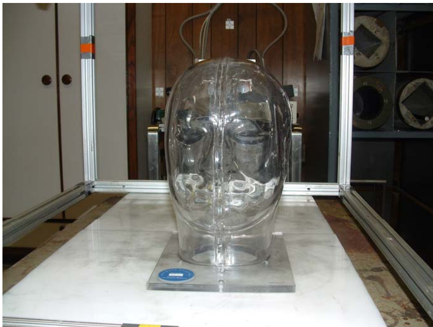
Figure 34: Head phantom used in the experiment. It will be filled with deionized water and placed upside down during the experiment.
