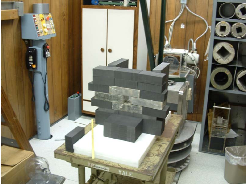
Figure 31: The 5 cm x 5 cm collimator made of four lead bricks (the brown colored in the center). The thickness of the collimator is 10 cm. The lead brick has a dimension of 20 cm x 10cm x 5 cm. The black bricks are graphite. The assembly is placed on a cart and between the assembly and cart is 10-cm thick polyethylene plate.
