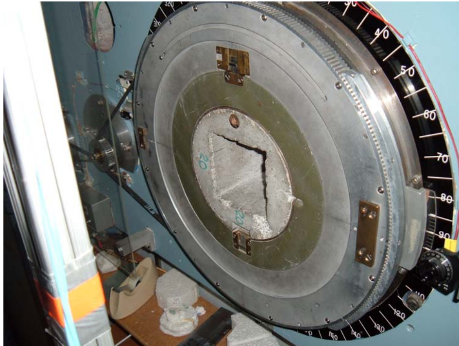
Figure 33: The standard 20 cm x 20 cm beam collimator used in the experiment.
