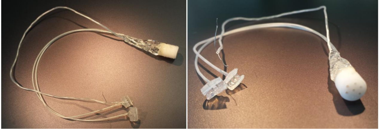
Figure 4.0.1: Two views of the same finished electrode. This is an example of an electrode with two bipolar cuffs and a bipolar EMG electrode in one package with a 6-pin PlasticsOne connector. It is ready for electrical characterization followed by gas sterilization in preparation for implantation on the sciatic nerve in the rat model.
